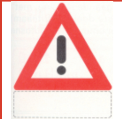
Danger. Details of the danger are shown on the plate beneath
