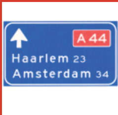
Low level motorway information sign showing both main and intermediary destinations and motorway number
