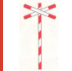
Level crossing with single track
