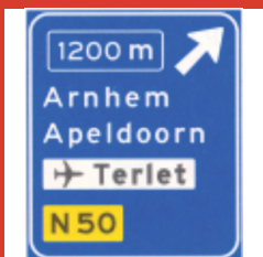
Advance warning sign of a motorway showing the distance to the next exit (the top destination is the name of the exit), direction to aerodrome/airport and the road number
