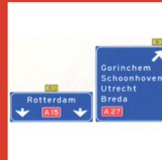
High level motorway information sign showing lane instruction for through traffic and exit panel showing intermediary destinations, with the motorway number and European route numbers
