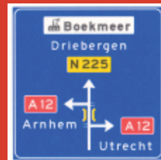
Non-motorway advance information panel showing intermediary destinations, road numbers, a viaduct symbol and a sign for an industrial zone
