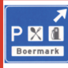
Information sign of exit to motorway service area, showing the name of the rest area and symbols for the services offered
