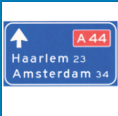
Low level motorway information sign showing both main and intermediary destinations and motorway number
