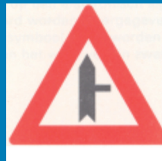
Road junction with priority over minor road from the right
