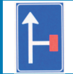
Advance warning of a no through road for vehicles
